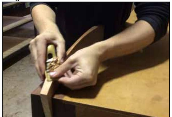
**23.** While the assembly is drying, shape and sand the back legs. The back legs are universal (no left and right). You can customise the back legs with a variety of details such as round-overs. If using a router bit with a bearing to do extra shaping, be careful that the bearing doesn't fall in the screw holes or the mortise. Note; the tapered screw holes are deliberate, to allow for the expansion and contraction of the back rest.
