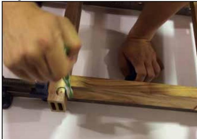
17. Once the glue used for the frame has set, you should now be able to glue on the front legs.
