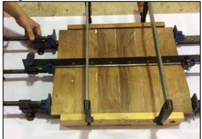
7. When tightening the clamps across the seat, ensure an even pressure top and bottom. The seat components have been machined square, but clamping with a pressure bias can induce cupping in the seat. It is a good idea to check with a straight edge to ensure that the seat is flat. There is no need to protect the outer ripple cuts from clamp damage, as these edges will be cut away later.
