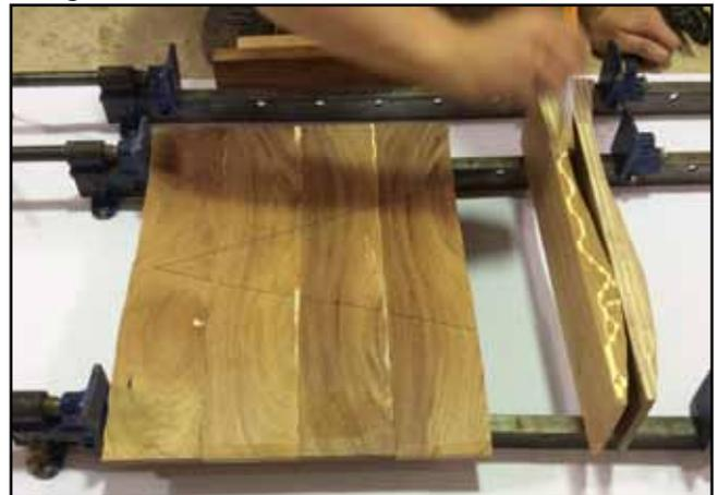
6. When fitting each component to the next, slide it back and forth a few times to transfer the glue from the applied surface to the dry surface. Ensure that the front of the components are even (this is really important!). It is ideal to clamp a pair of cauls across the front and back of the seat, as this will ensure that the seat is even. **(Image 5)**
