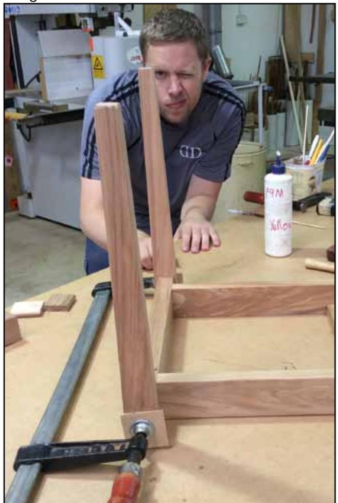
**20.** While the front legs are setting, you can shape the back support. When fitted at the specified height relative to the seat, the curve cut into the face of the back support will give you a good ergonomic solution for the chair. Any discretionary shaping you choose to do should avoid radically altering this curve. Be aware of how the grain of the back support blank works visually with your intended shape.
